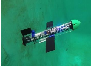
Fig. 1. The assembled glider mid-mission rising while set in the pause time mode.
